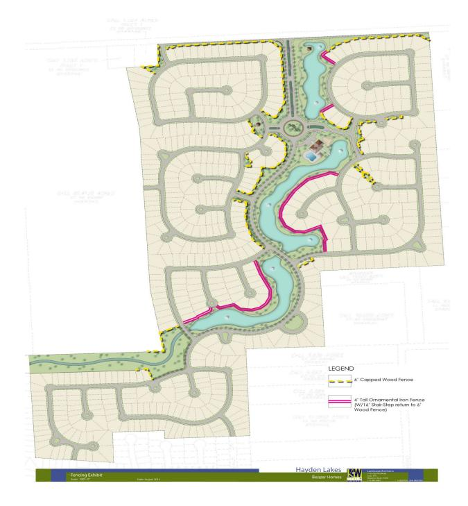
Yellow - Type b. 6' Upgraded Wood Fence with Cap Rail Pink - Type d. 4' Steel or Wrought Iron Fence
